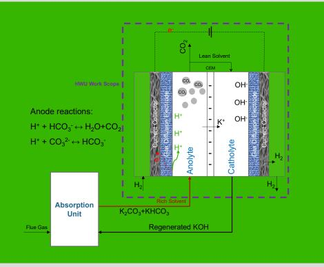
A schematic of the pH-swing electrochemical regeneration system that has been modeled by HWU in the DRIVE project
